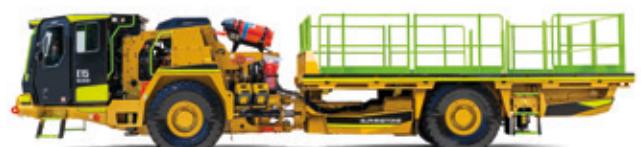
Optional guardrail system with optional self-closing gate.
