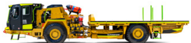
Two-Piece Deck, Crane-Ready, combined 5.2m x 2.5m [17' x 8'2"].
