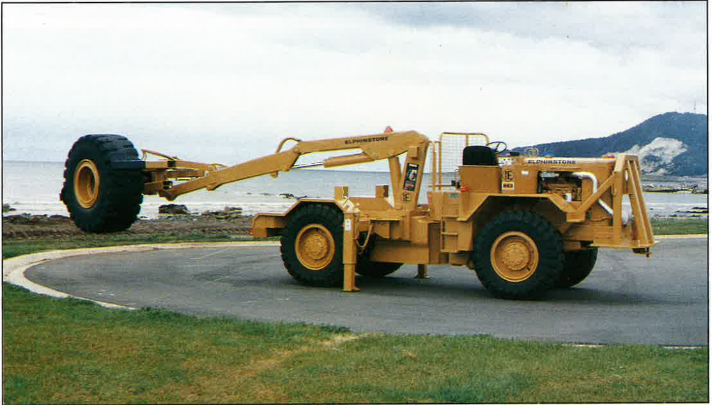
ELPHINSTONE 923 TYRE HANDLER Alternative Tyre Size Clamps Available.
