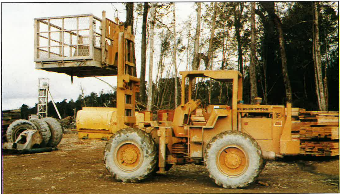
ELPHINSTONE U.F. 4000 FORK LIFT TRUCK (Shown with Service Basket) Capacities from 3000 to 5000 kg.
