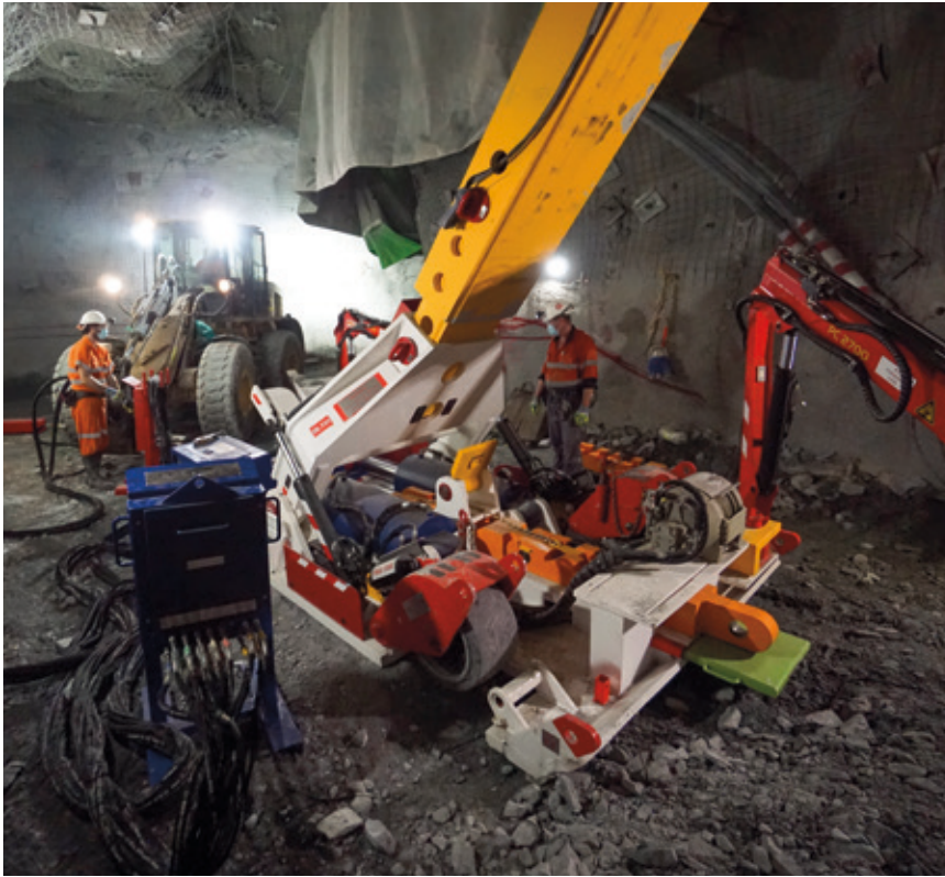
7. The control station and hydraulic hoses are moved into position and connected. In this case the auxiliary implement controls on an IT loader are used to operate the MED.
