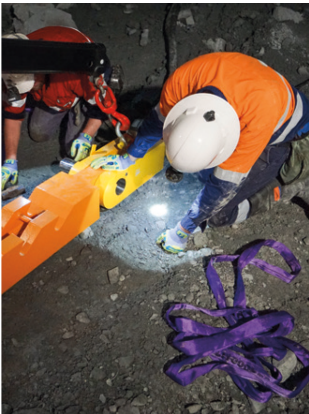
13. The connecting link is secured to the pulling rack using the load pin.
