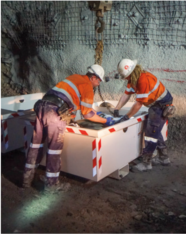
4. The connecting racks are attached to the machine using D-shackles and slings.
