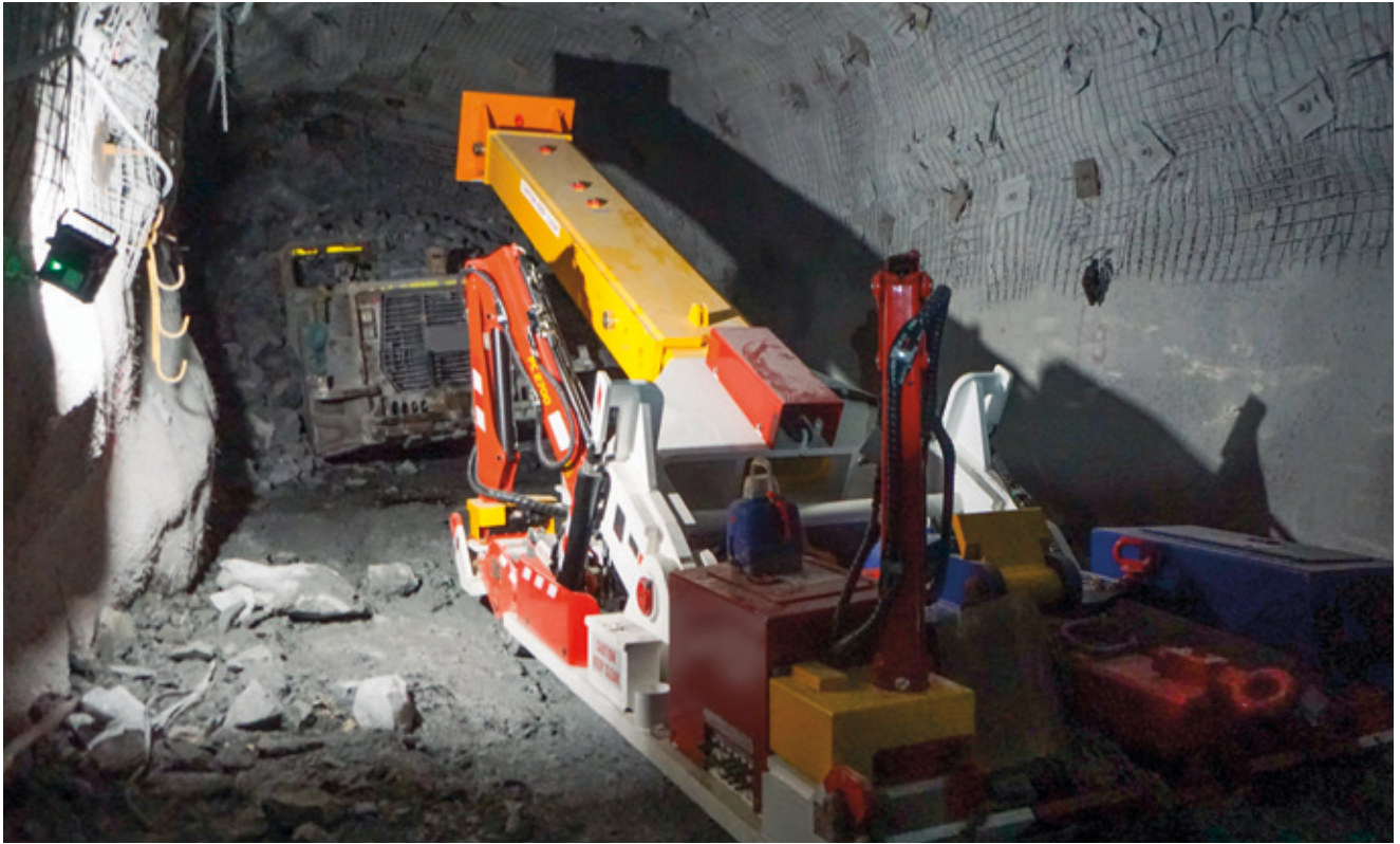
1. MED360 is being moved into place following the preparation of a solid and level base before the extraction commences.
