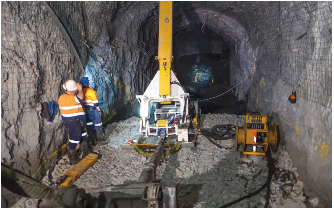
5. The connecting racks are attached to the machine using D-shackles and slings.
