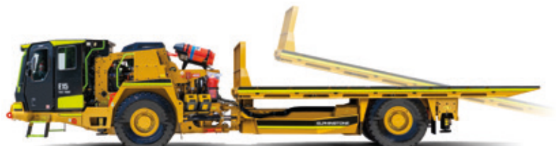
E15 Tilt Tray | 6m x 2.5m (19'8" x 8'2") Rear chassis increased by 900mm (35")
