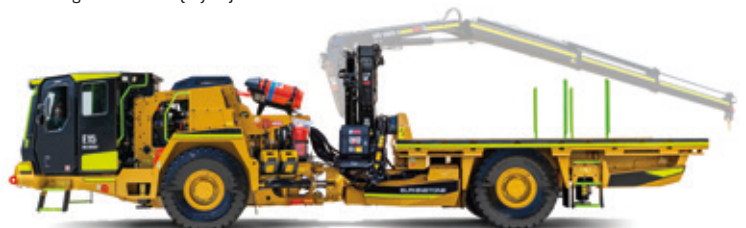
E15 Delivery | Integrated Crane with 4.5m x 2.5m (14'9" x 8'2") Heavy Duty Deck
