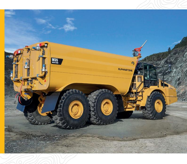
Designed to fit a Caterpillar 740C, 745C and 745
