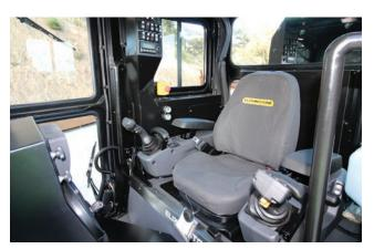
The dash includes gauges for engine coolant temperature, articulation, voltage and fuel level. Hour meter, speedometer and tachometer are standard. All major systems are monitored by warning lights. Both doors are fitted with interlocks and seat belt alarms are visual and audible.
