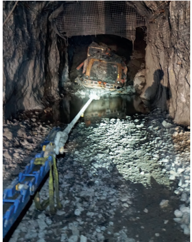
7. As the pressure is increased the machine is released from the fallen debris.
