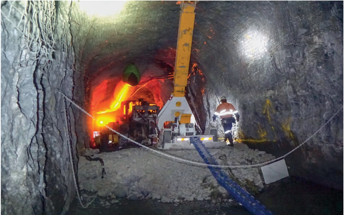
4. The engineered racks are assembled and pulled through the MED using the winch.
