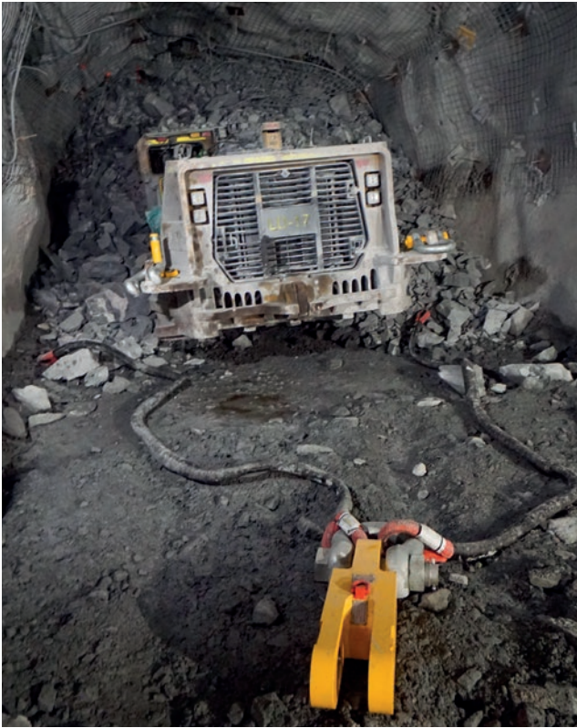
11. Tow slings have been secured to the connecting link.
