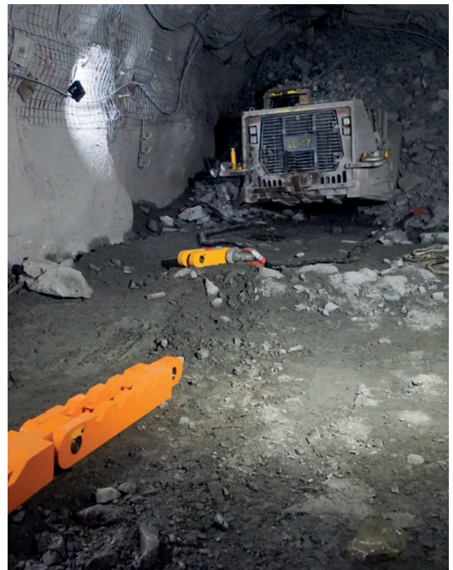
10. Tow sling is secured to the buried asset using rated 'D-shackles' and tow slings.
