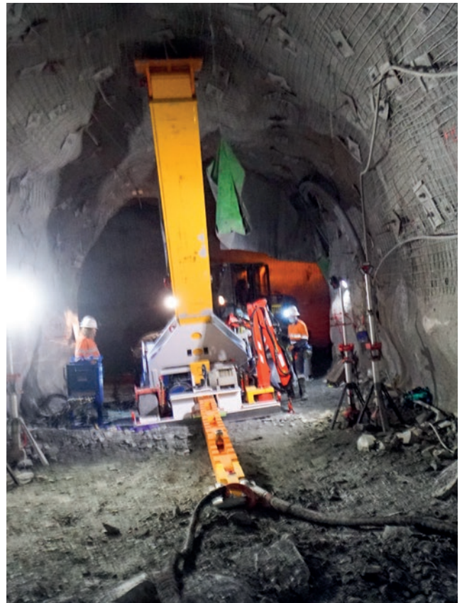
14. The MED360 is ready to commence the bedding in process and subsequent extraction.
