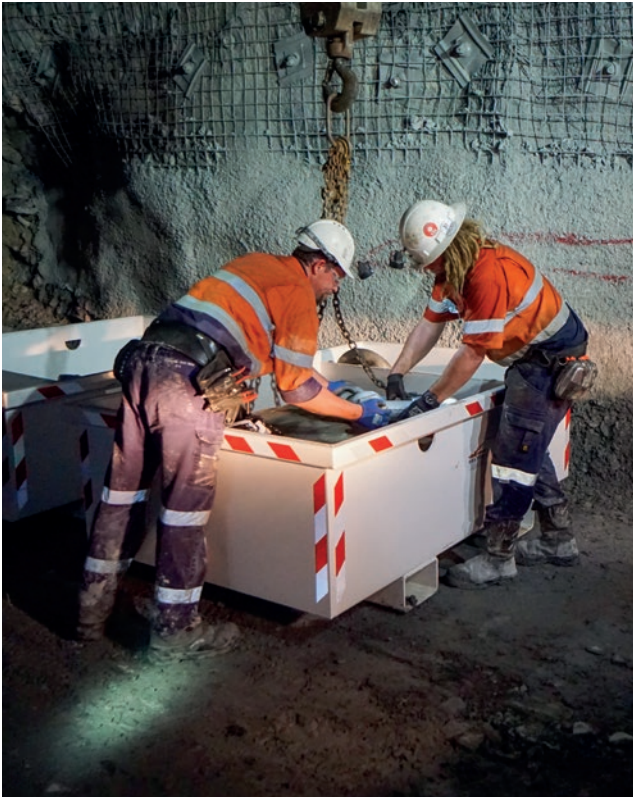
4. Correctly rated 'D-shackles' provided with the MED360 are prepared to attached to the buried asset.
