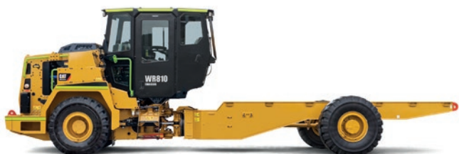
WR810 Cab Chassis: Base chassis provisioned for the installation of modules for specific applications.
