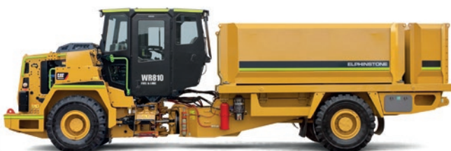
WR810 Fuel: Provides bulk transport of fuel underground to storage tanks or can be used for in situ filling of production machines minimising down time.
