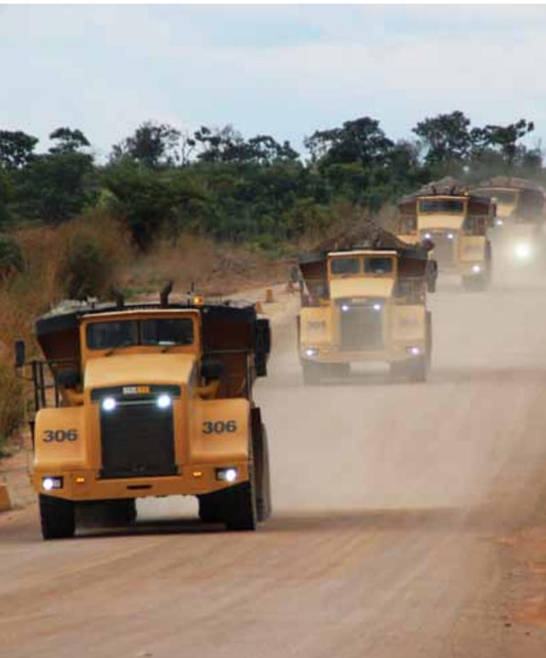
With a narrow design that allows for use on haul roads around 15 metres (49 feet) wide, the Haulmax 3900 Series Truck was developed to operate on cycles of approximately 50km (30 miles). Simply put, narrower roads cost considerably less to build and maintain, the longer the distance, the larger the cost saving.
