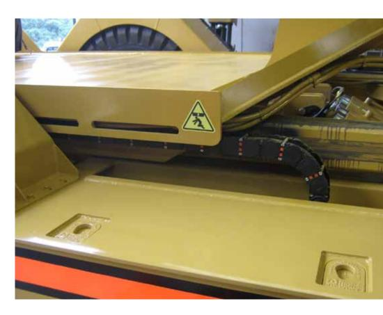
Tilting/Sliding Tray. The tilt tray is equipped with hydraulic extension cylinder so slide the tray and telescoping hydraulic cylinders to tilt the tray.
