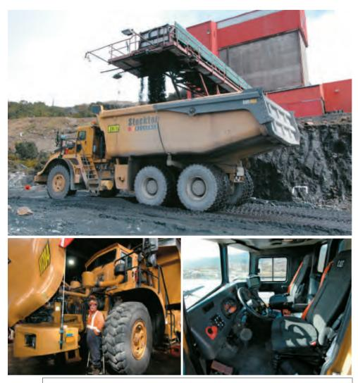
*Top*: Automated loading at Station 2 means driver doesn't have to leave cab, a boon in Stockton's often-challenging weather
