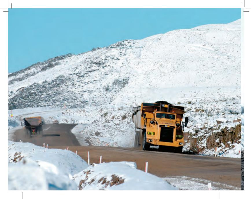
The Stockton mine's main haul road, the "2 to 5," drops 400 metres along its 7.5km length. The Haulmax 3900's rear brake swept area of over 10 square metres keeps 130 tonnes all up well under control on the downhill run
