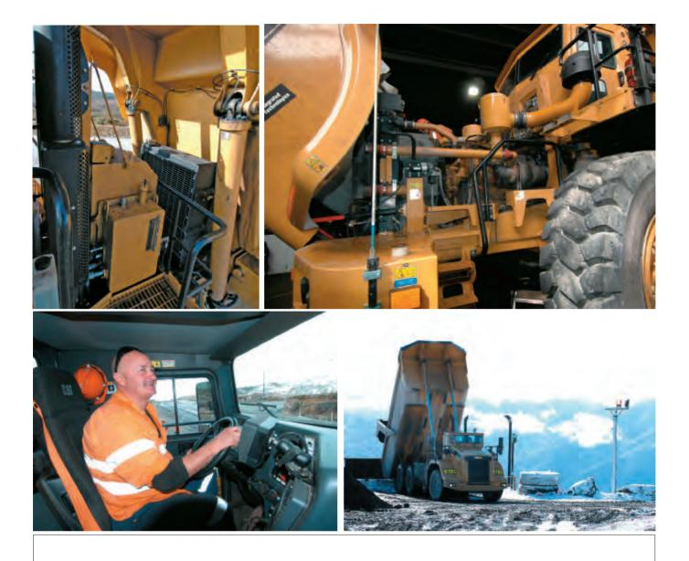
*Top left*: Supplementary air/oil radiator soaks up heat from brake-based automatic retarder system *Top right*: Providing safe and easy access around engine and various maintenance points has been a priority for Haulmax designers *Above left*: Driver Lockey Mundy "felt like a bit of change," so swapped the cockpit of a topdresser for the cab of a mining dumptruck *Above right*: Twin hydraulic rams raise the Haulmax's massive body quickly and smoothly
