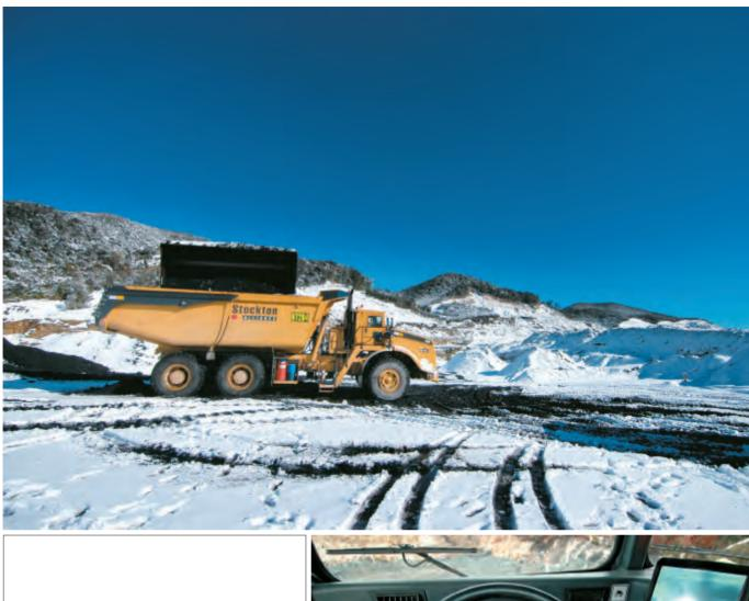
*Above*: The snow is beginning to get churned up as another truck is loaded. Note the simple chain tailgate lift on the Haulmax
